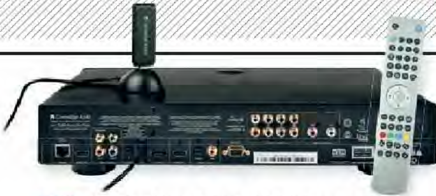
ABOVE: Left to right - Ethernet and secondary HDMI ports, component/composite video, USB (here with wireless receiver), e-Sata port, primary HDMI out, opt/coax digital audio and 7.1 channel plus stereo RCA analogue audio outputs
